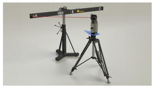
Laser trackers have been widely used in industry for over two decades. From their original design in the late 1980's, trackers have been well accepted and adopted into the metrology workspace. The combination of industry needs and R&D innovations has created a recipe for some really cool advances in the technology—advances which push the accuracy envelope, improve the flexibility and ease of use, and lower the costs of ownership.
