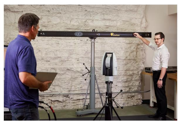
**Applying the new ISO testing process,** the ISO-10360-10:2021 Annex E, is Brunson's Lead Mechanical Engineer Tyler Santoro (right), as Brunson Director of Engineering Mark Meuret observes. The recently approved Annex E interim testing procedure is similar to the earlier NIST IR-8016 process.
